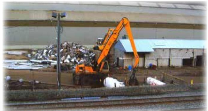
*One of the model 934 Liebherr cranes used to sort scrap metals*
